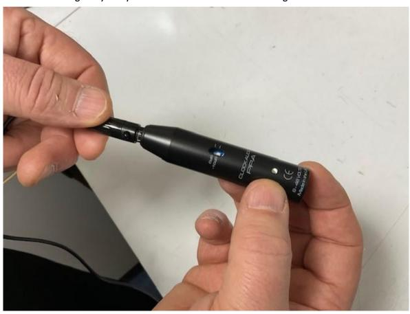
When plugging in the microphone mini XLR to the phantom module be very careful to offer the mini XLR into the socket and turn very gentle until it slides into the socket. The mini XLR does not plug in line with the phantom unit as you would expect. It should not take any effort in insert.
